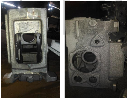
Fig 4:6 Visual Inspection: Sand Inclusion
